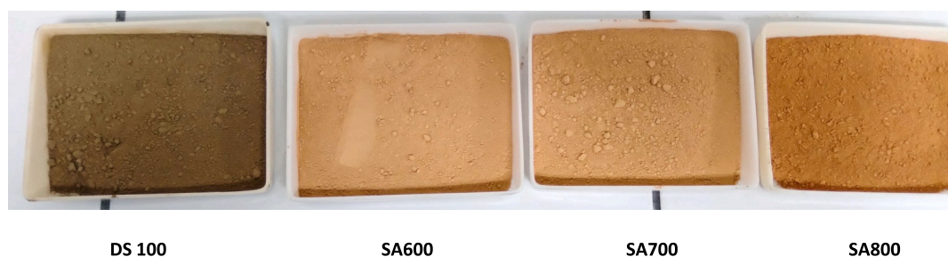
Fig. 1. Appearance of dried (DS100) and calcined (SA600, SA700, and SA800) water treatment sludge after grinding.
