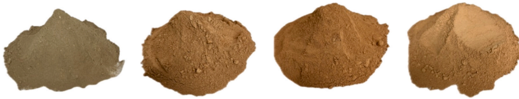
Fig. 1. From left to right: the appearance of the WS100, WA600, WA700 and WA800 treatment sludge after machining.
